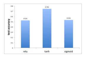
tanh function has the highest test accuracy. Therefore, we chose tanh function in our best model. An insight that we got from piazza is that ReLU and sigmoid both saturate at 0 on the negative side, whereas tanh saturates at -1. Thus, if a weight gets multiplied by the output of a tanh, the size of the weight matters for negative values of the input to the tanh. It does not matter for any negative ReLU inputs and for sufficiently large sigmoid inputs in absolute value. [7]
