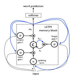
Figure 3: LSTM unit and its gates
