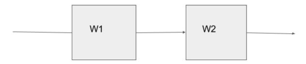
Version C: A sequential RNN or LSTM network with one set of matrices but skip connections skipping every two. Thus the equations alternate between the following. First h(t) = Relu(W1\*h(t-1) + Wx\*Input). Then h(t) = Relu(W1\*h(t-1) + Wx\*Input) + h(t-2)
