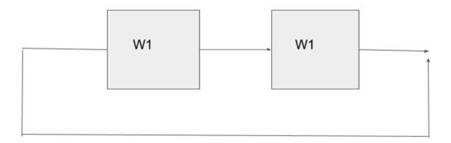
Version D: Two sets of matrices with skip connections over every two blocks. Thus the equations alternate between the following. First h(t) = Relu(W1\*h(t-1) + Wx\*Input). Then h(t) = Relu(W2\*h(t-1) + Wx\*Input) + h(t-2)
