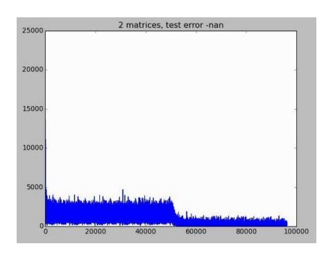
Version C: Same task but we see that the neural network with skip connections is doing very well in learning the task! Nearly after one epoch we are getting close to zero mean squared error. In addition there were no difficulties with this network giving NaN values. It is possible that skip connections have less exploding gradients!
